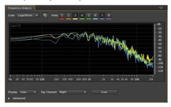
For a selected file (or portion of a file) in the Waveform Editor, this panel shows amplitude response (vertical axis) plotted against frequency (horizontal axis). The frequency range can be displayed linearly or logarithmically; you can store up to eight "snapshots" taken at particular points in the waveform, and for comparison, display each one using a separate color.
