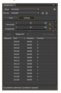
This panel is the same as the one that opens when you select part or all of a waveform in the Waveform Editor, then choose Effects > Diagnostics. It provides processing that can minimize clicks and clipping, as well as delete silence and show marked sections of a waveform.
